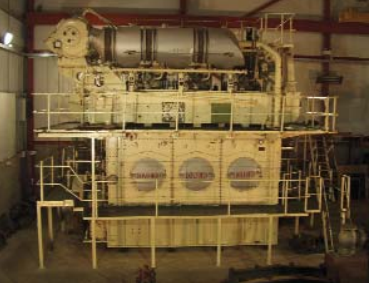
The Doxford marine oil engine at the Regional Museum Store. © / Photographer: Tyne and Wear Museums
