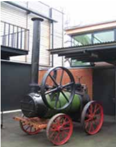
Clayton & Shuttleworth portable steam engine Photographer: William Phillips © Museum of English Rural Life
